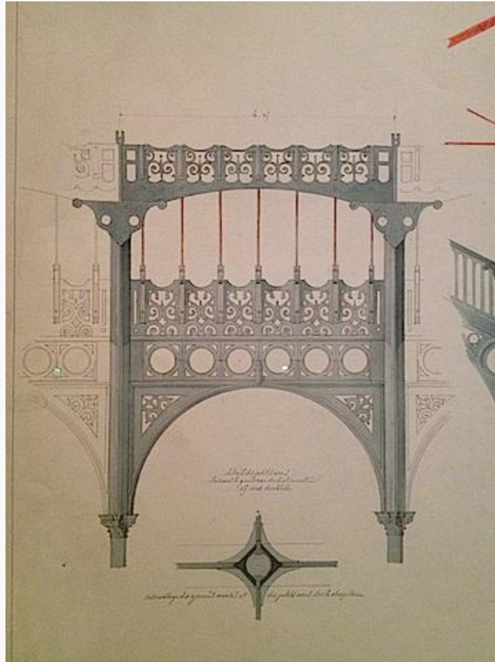
Fig. 12, Henri Labrouste, Bibliothèque Sainte-Geneviève: Study of the cast-iron trusses of the upper floor and of the iron roof trusses , 1846. [return to text]
