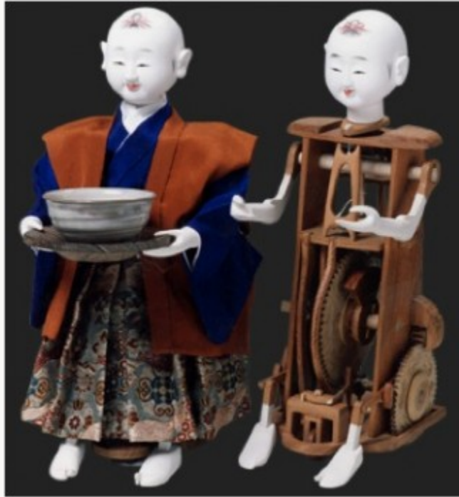
Fig. 7, Tea-serving mechanical doll , 19th century. Metal, cloth, wood, and gofun. [return to text]
