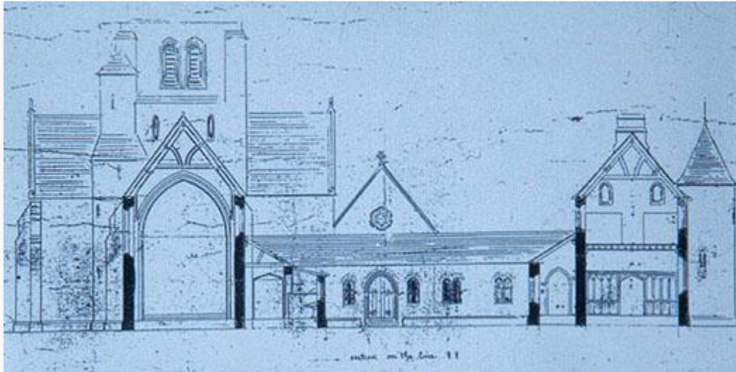
Fig. 3, A. W. N. Pugin, North/south section looking at Chapter House façade, Mount Saint Bernard Abbey. (Courtesy of the monks of Mount Saint Bernard Abbey) [return to text]
